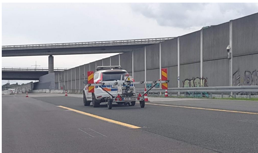
Figure 6 VTI-XPS, reference for transversal evenness and crossfall. Photo: Thomas Lundberg, VTI.
