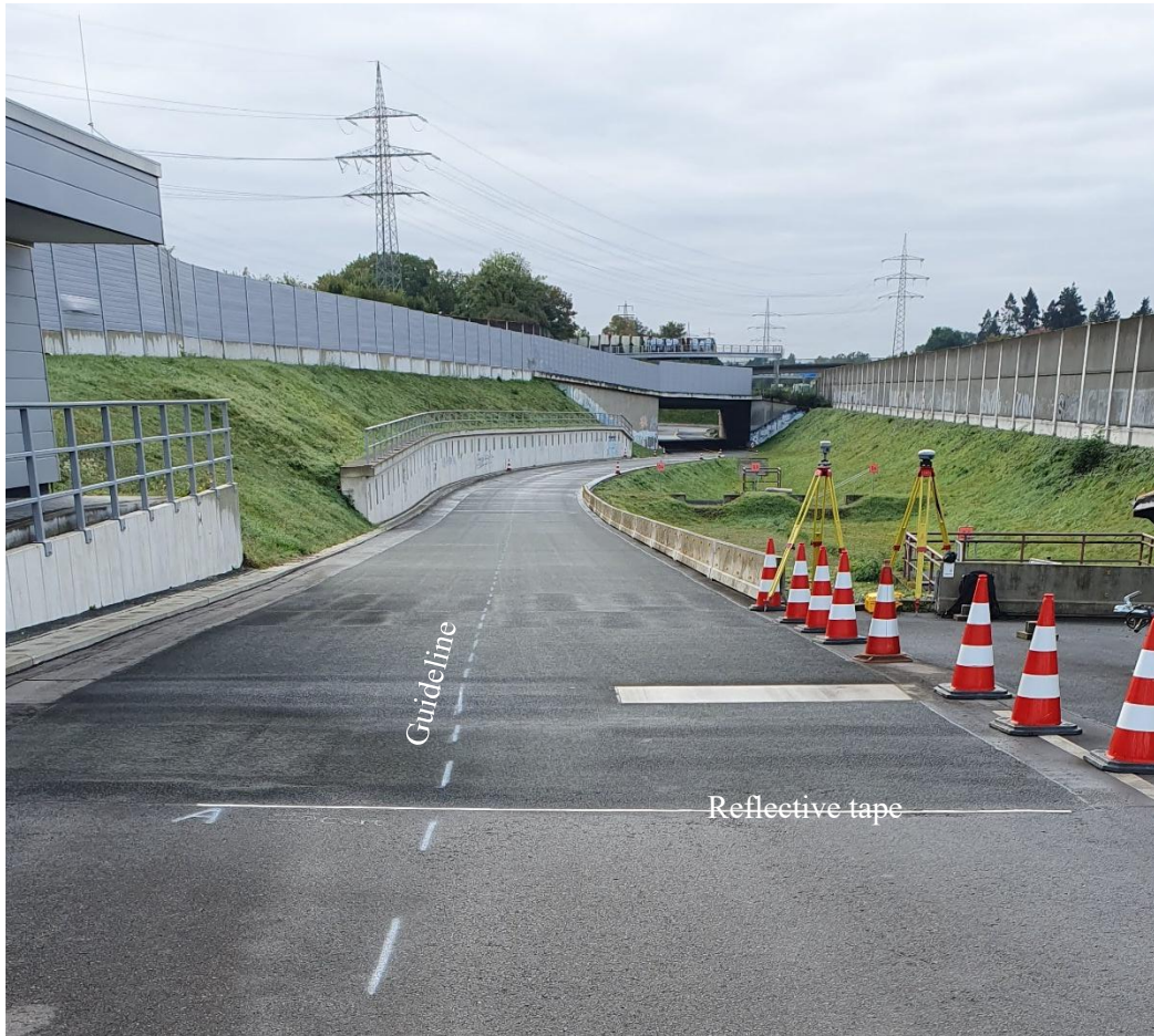
Figure 12 Reflective tape at the start of section A and the guideline for transverse assistance for the driver. Photo: Nicklas Mattisson, VTI.
