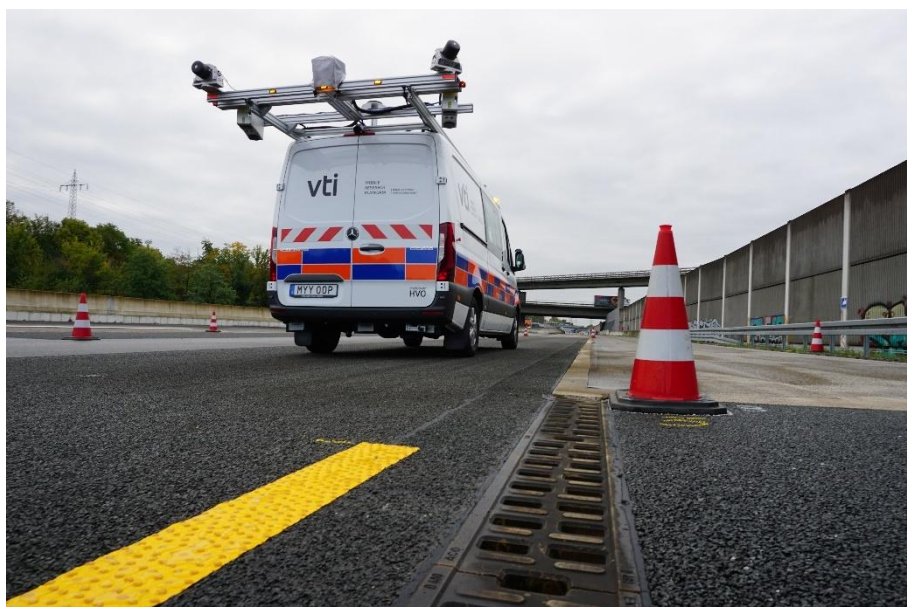
Figure 8 Reference equipment VTI-MRP for Megatexture. Photo Nicklas Mattisson, VTI.
