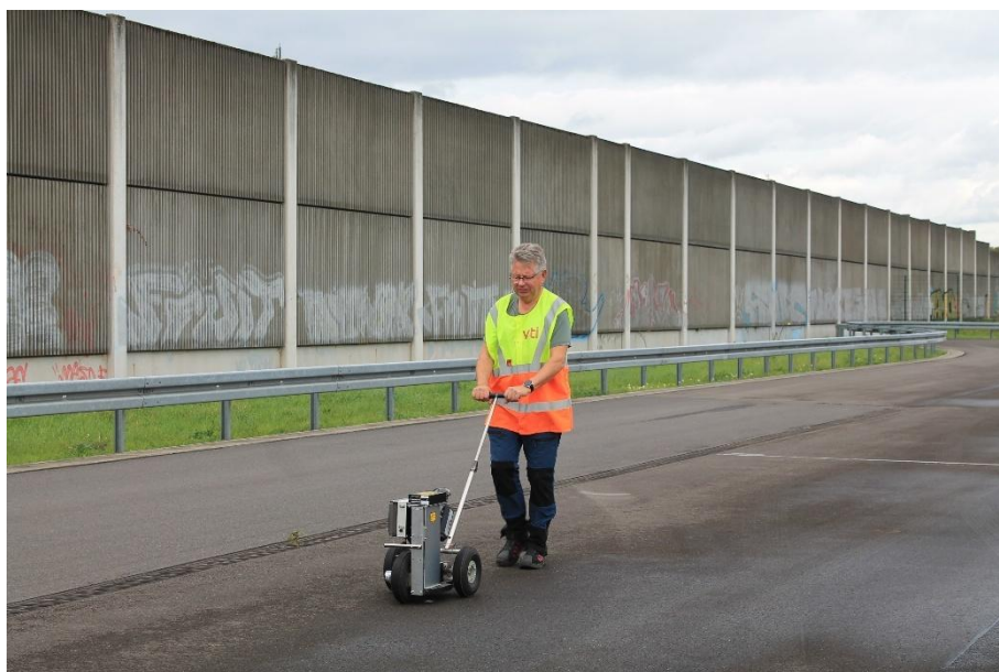
Figure 7 Reference equipment VTI-PTT for macrotexture profile measurements. Photo: Linda Corper, VTI.
